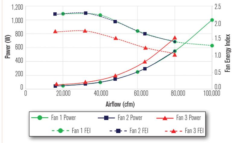
large-diameter fans aggregates performance at the maximum and part-load airflow settings inherent to the fan. For comparing performance of fans at a given airflow point, designers may have to look beyond the DOE metric. Soon, in addition to data determined using the DOE test method, engineers will be able to use AMCA 208 to determine FEI and have applications data from ASHRAE Standard 216P testing to guide ceiling-fan selection and application.
